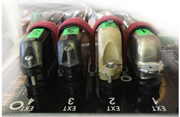
Fig. 9 – Four amphenols restrained with Velcro strips.
