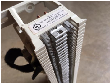
Fig. 51 – Bridge clips on a 66 block.
