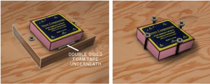
Fig. 31 – PowerDSINE mounting techniques: foam tape (left), or screw constellation (right)
