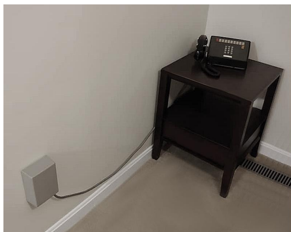
Fig. 57 – 66E3-25 wall installation with decorative cover for a 2830 desk set.
