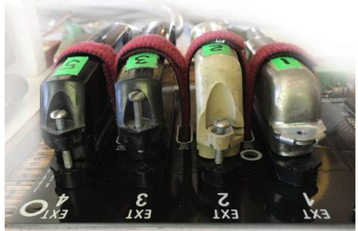
Fig. 9 – Four amphenols restrained with Velcro strips.
