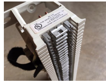
Fig. 52 – Bridge clips on a 66 block.
