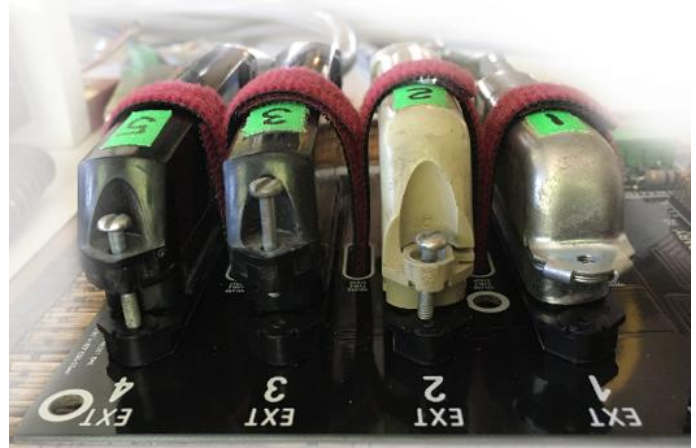
Fig. 9 – Four amphenols restrained with Velcro strips.
